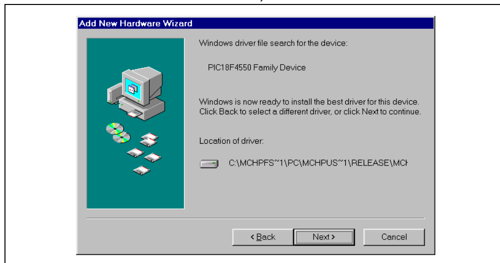
FIGURE 2-3: HARDWARE WIZARD, READY TO INSTALL DRIVER
